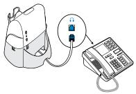
Connect the audio cable included with and pre-attached to the headset base to the headset port on telephone.
